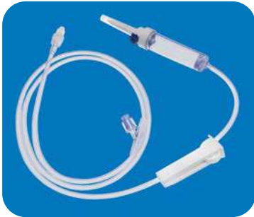
Gravity IV Set Standard IV set for infusion of drugs and liquids Drip Chamber, 20drops/ml, filter 15um Roller Clamp Needle Free Valve Male Luer Lock
